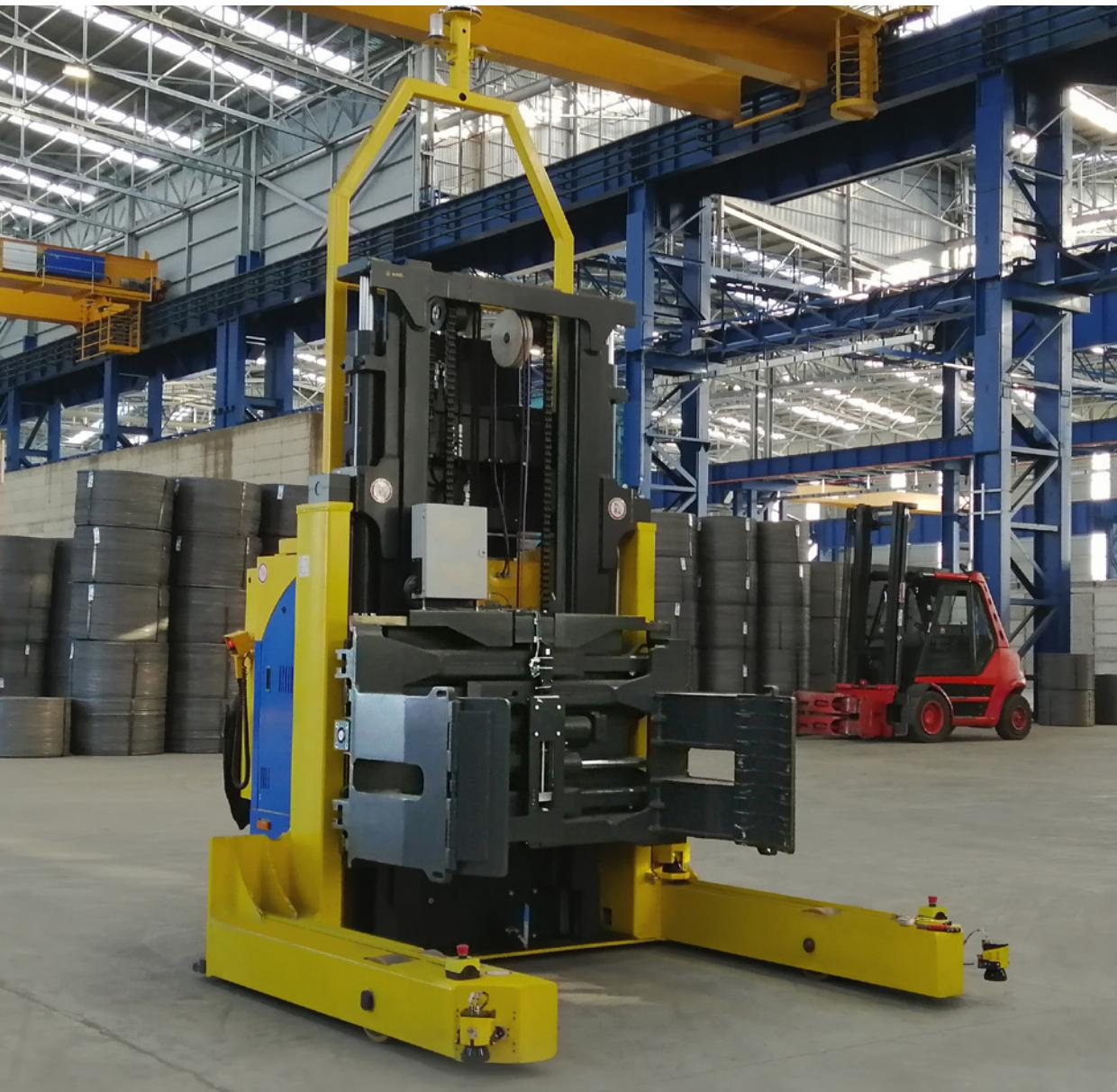
Triplex Mast with Double Fork Positioner for AGV Machines
